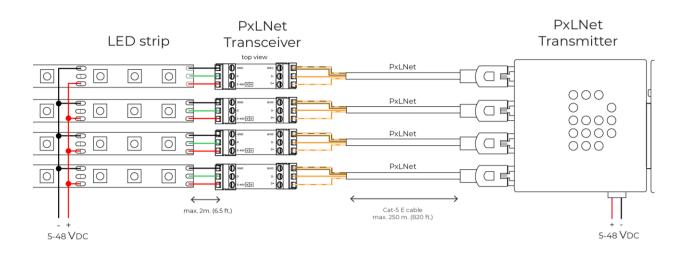
DiGidot C4 with PxLNet Transmitter connected by Cat-5E network cables which are soldered to PxLNet Transceivers which are soldered directly to a pixel controlled LED product.
