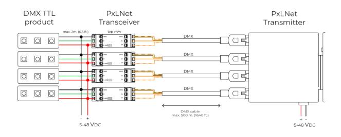
Using an external DMX signal, connected to a PxLNet Transceiver which is connected to a DMX TTL controlled LED product. The DMX signal can be soldered, as indicated in the drawing or can be inserted in the RJ45 bus on the top side (DMX pinout according to USITT standard, see page 5)
