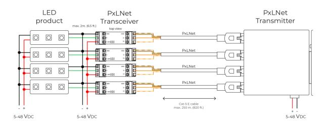
DiGidot C4 with PxLNet Transmitter connected by Cat-5E network cables to PxLNet Transceivers which are soldered directly to a pixel controlled LED strip. At the end of every LED strip another PxLNet Transceiver is placed in transmit mode, to send the remaining signal to the next LED strip. Please note that the operating mode jumper [4] on the top side must be removed to change it to transmit (Tx) mode.
