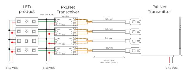
DiGidot C4 with PxLNet Transmitter connected by Cat-5E network cables to PxLNet Transceivers which are soldered directly to a pixel controlled LED strip. At the end of every LED strip another PxLNet Transceiver is placed in transmit mode, to send the remaining signal to the next LED strip. Please note that the operating mode jumper [5] on the top side must be removed to change it to transmit (Tx) mode.
