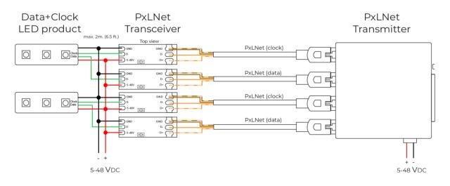
DiGidot C4 with PxLNet Transmitter connected by Cat-5E network cables to PxLNet Transceivers which are soldered directly to a pixel controlled LED strip which is powered from an alternative section.
