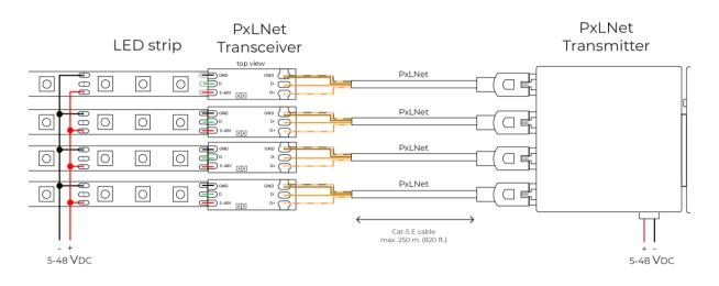
DiGidot C4 with PxLNet Transmitter connected by Cat-5E network cables which are soldered to PxLNet Transceivers which are soldered directly to a pixel controlled LED product.
