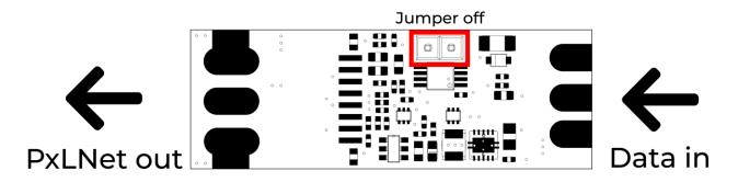
Remove the jumper [7] as indicated, to activate transmit (Tx) mode.
