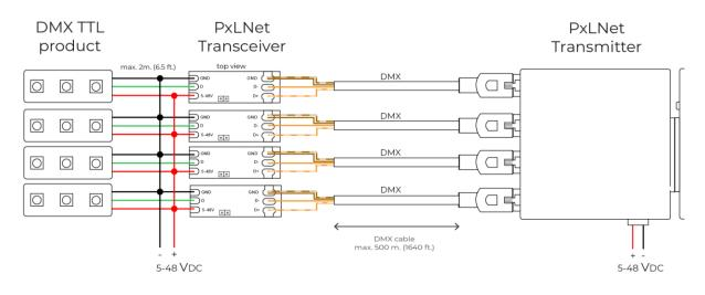
Using an external DMX signal, connected to a PxLNet Transceiver which is connected to a DMX TTL controlled LED product. The DMX signal can be soldered, as indicated in the drawing or can be inserted in the RJ45 bus on the top side (DMX pinout according to USITT standard, see page 5)
