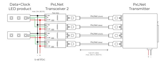
DiGidot C4 with PxLNet Transmitter connected by Cat-5E network cables to PxLNet Transceivers which are soldered directly to a pixel controlled LED strip which is powered from an alternative section.
