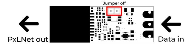
Connect a network cable to the RJ45 bus and connect it to the next PxLNet Transceiver in receiving mode (Rx).
