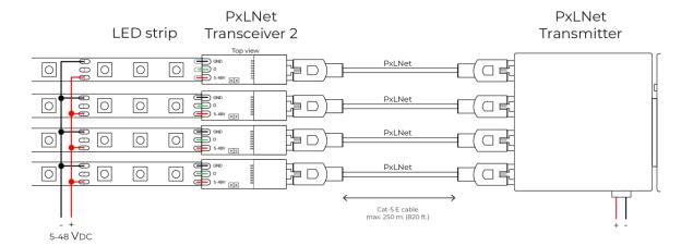
DiGidot C4 with PxLNet Transmitter connected by Cat-5E network cables which are soldered to
