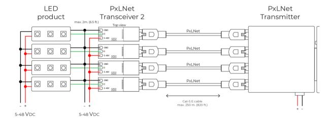
DiGidot C4 with PxLNet Transmitter connected by Cat-5E network cables to PxLNet Transceivers which are soldered directly to a pixel controlled LED strip. At the end of every LED strip another PxLNet Transceiver is placed in transmit mode, to send the remaining signal to the next LED strip. Please note that the operating mode jumper [5] on the top side must be removed to change it to
