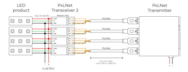
PxLNet Transceivers which are soldered directly to a pixel controlled LED product.
